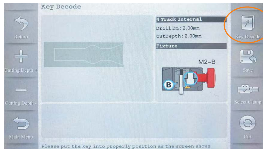
6) Select proper clamp, then click on 'Key Decode', probe will be detected many different points of whole key.
