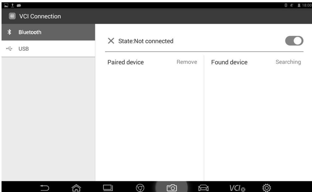
2. After approximately one minute, you can search for the ID of the VCI box connected to the vehicle. Click Connect to pair.
