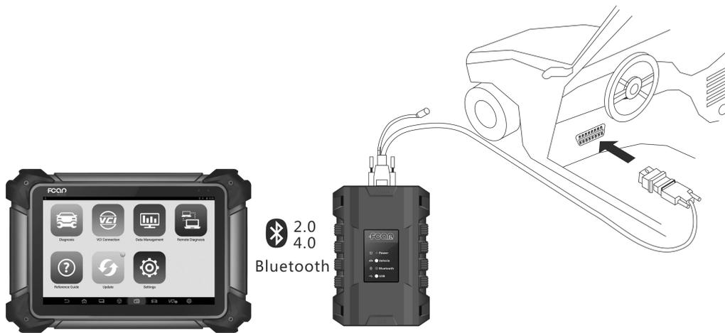
Then turn on the machine, enter [Settings]-[VCI connection]. It can be connected via Bluetooth and USB cable:
