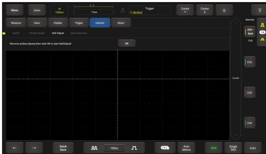
Tap **OK** on the pop-up message box to start calibration. The LED on the Scopebox starts flashing and the prompt message “Self Adjust is running” will appear on the upper left corner of the screen.
