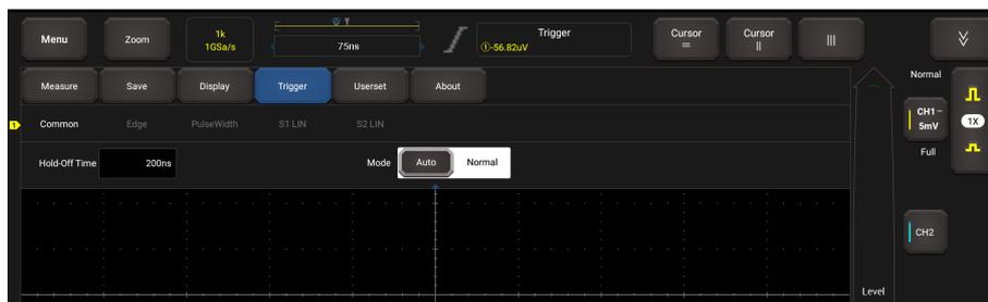
Auto: It allows the Scopebox to acquire waveforms even when it does not detect a trigger condition. If no trigger condition occurs while the Scopebox is waiting for a specific period, it will force itself to trigger. When forcing invalid triggers, the Scopebox can not synchronize the waveform, and then waveform seems to roll across the display. If valid triggers occur, the display becomes stable on the screen.
