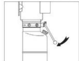
**Warning:** *Always make sure safety latches on both sides clear the rack at same time when pulling down the release handle by adjusting the cable.*
