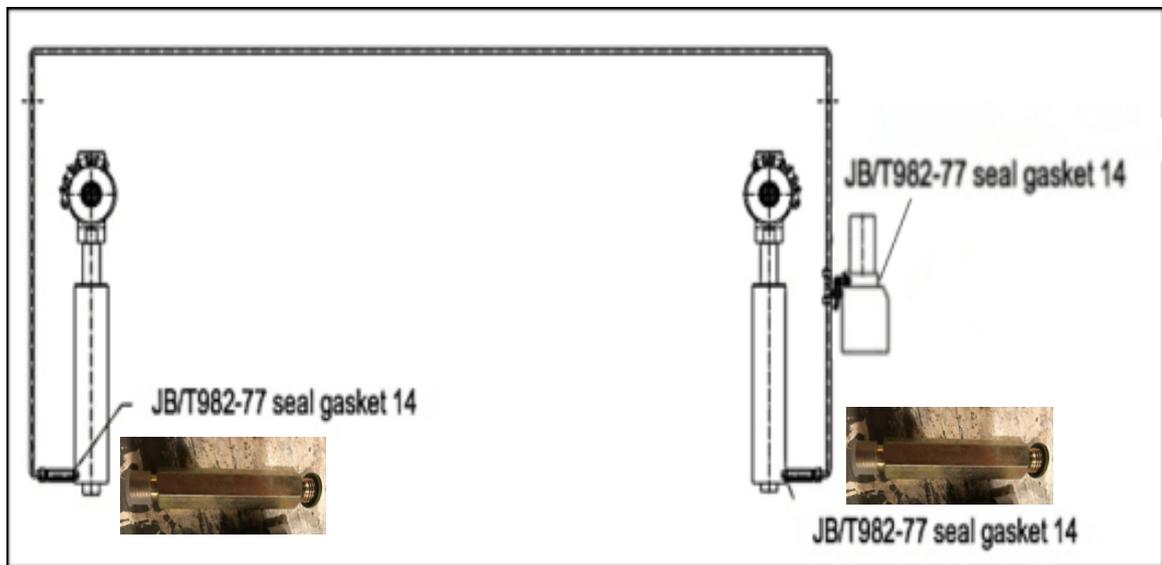
**Diagram of hydraulic line of base frame 2-post lift**
