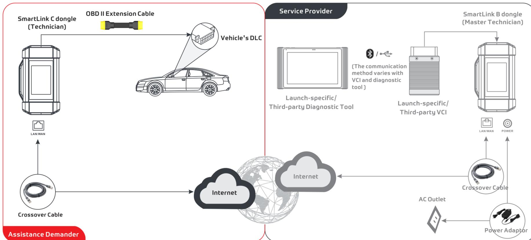
\* During the remote diagnosis, please do not disconnect the vehicle and the network (the network broadband of 100Mb and above is recommended). In addition, a SmartLink C dongle can only receive one remote diagnosis operation at a time.
