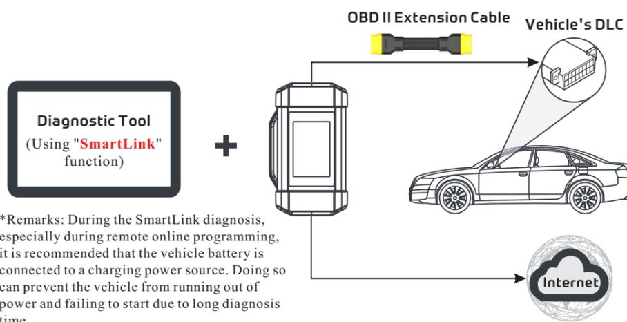
**\*Remarks:** During the SmartLink diagnosis, especially during remote online programming, it is recommended that the vehicle battery is connected to a charging power source. Doing so can prevent the vehicle from running out of power and failing to start due to long diagnosis time.
