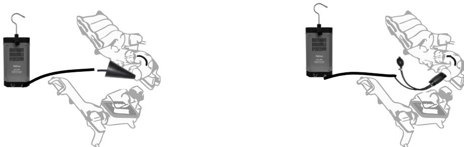
5. Connect Power Cords to 12V vehicle battery. For best performance, the vehicle battery shall be fully charged. Do NOT use a DC12V switch power supply.
